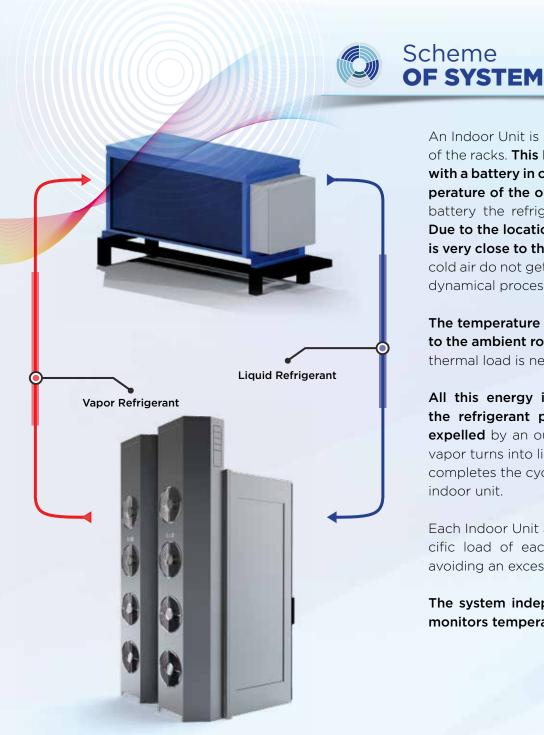
An Indoor Unit is screwed in the rear part of the racks. This Indoor Unit is equipped with a battery in order to reduce the temperature of the output hot air. Inside the battery the refrigerant turns into vapor. Due to the location of the battery, which is very close to the hot point, the hot and cold air do not get mixed and the thermodynamical process is very efficient.
